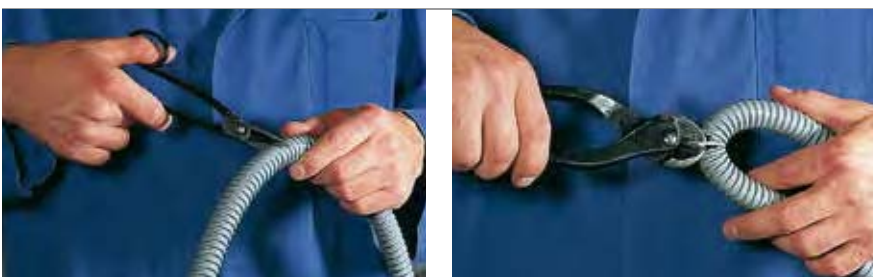
Kunststoff-Ummantelung durchschneiden Cut through the plastic sheathing
